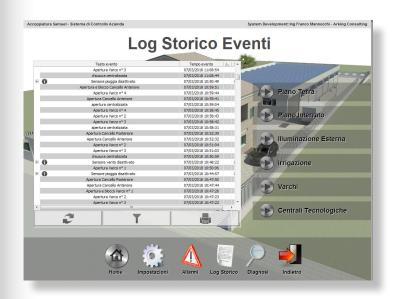
The project used Movicon 11 to manage home and building automation and it runs on 2 dedicated machines with Windows 10 operating system and IP65 capacitive touch-screen.
