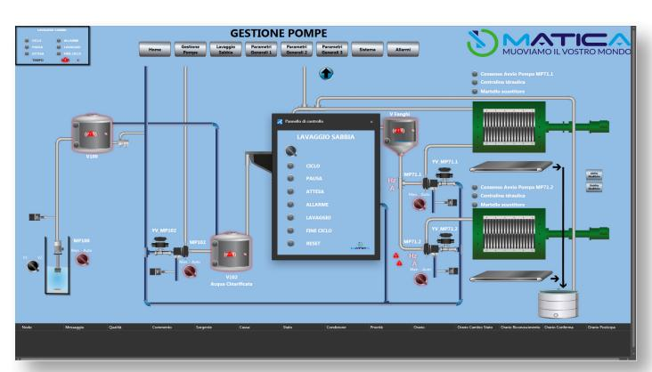
The homepage has been designed to limit the changing of the pages needed for the normal use of production processes, safeguarding the method of interaction now consolidated between the operator and the interface. The shortcuts associated to the mouse keys were kept the same as before.
