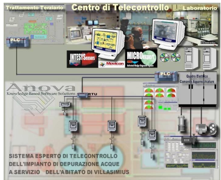
The main page of the remote control system at the Villasimius water purification plant created with the Movicon Scada from Progea.
